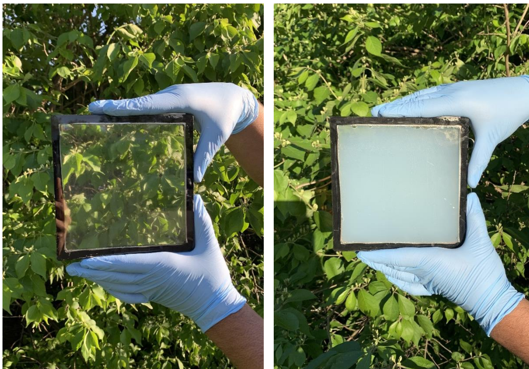
Figure 22 Model thermochromic window demonstration a) without sunlight exposure b) after exposure to solar radiation
