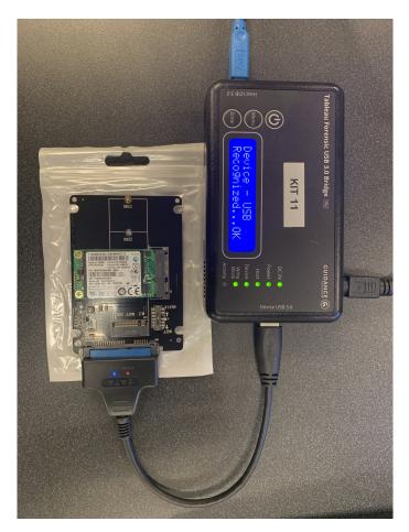
Figure 3.1. Laptop storage drive with USB write blocker
