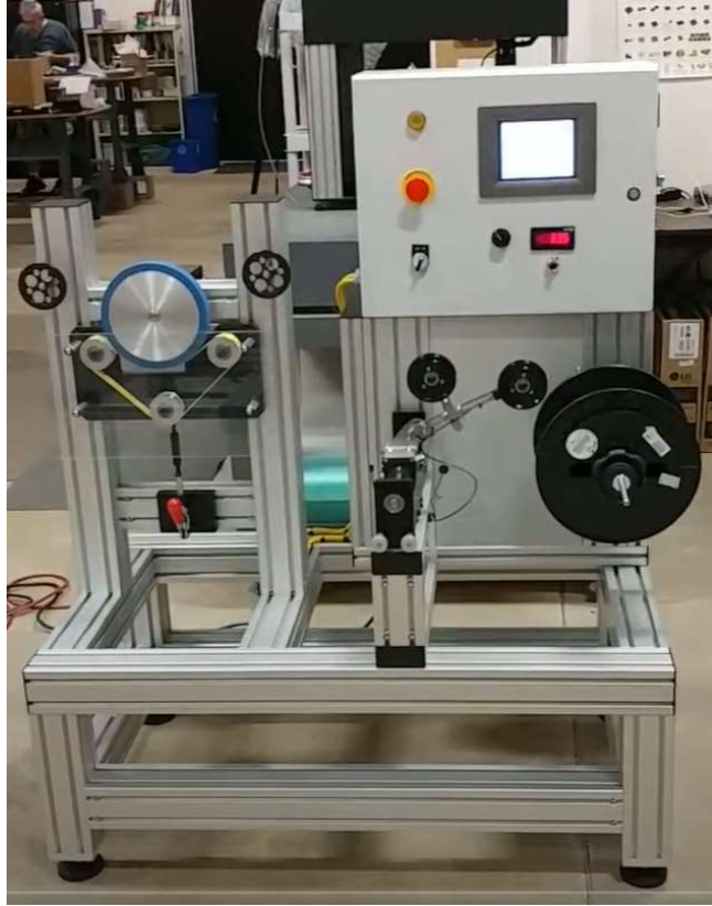
Figure 4.3 Capstan-driven servo motor proposed for improved control and repeatability of ultra-low feed rates necessary for the plasma treatment profiles under investigation.
