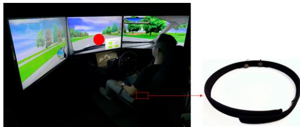
Figure 4.1. Experimental devices and setup (featured: miniSim (left) and C-2 Tactors (right))
