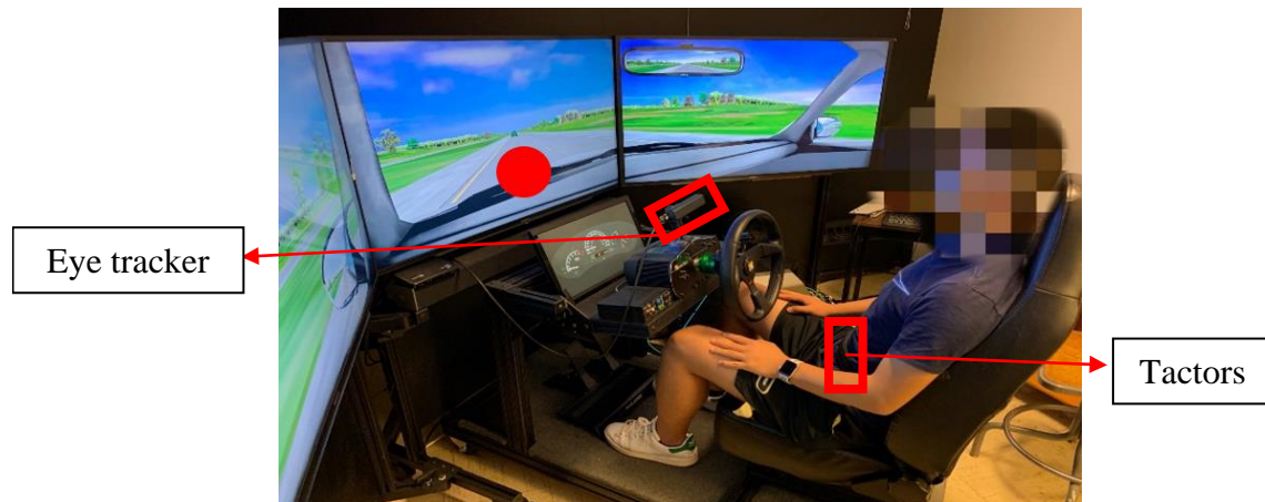
Figure 3.1. Experimental setup and devices (featured: NADS driving simulator, Fovio eye tracker, and C-2 Tactors)
