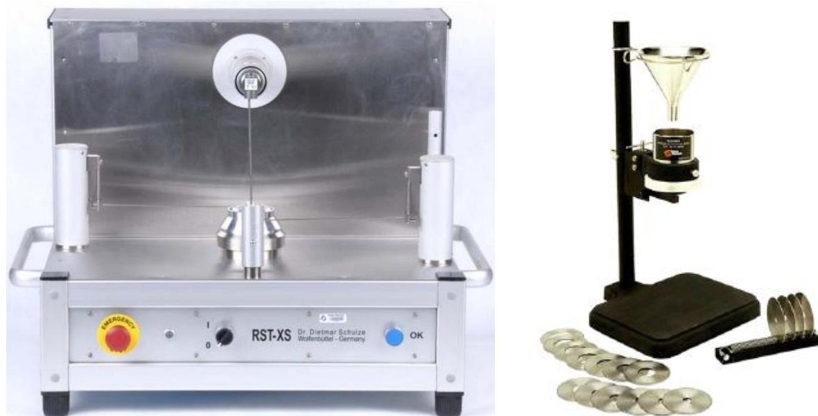
Figure 2.4: Schulze ring shear cell tester RST-XS (left) and Hanson Research's Flodex tester (right) (Hanson Research Corporation 2004)
