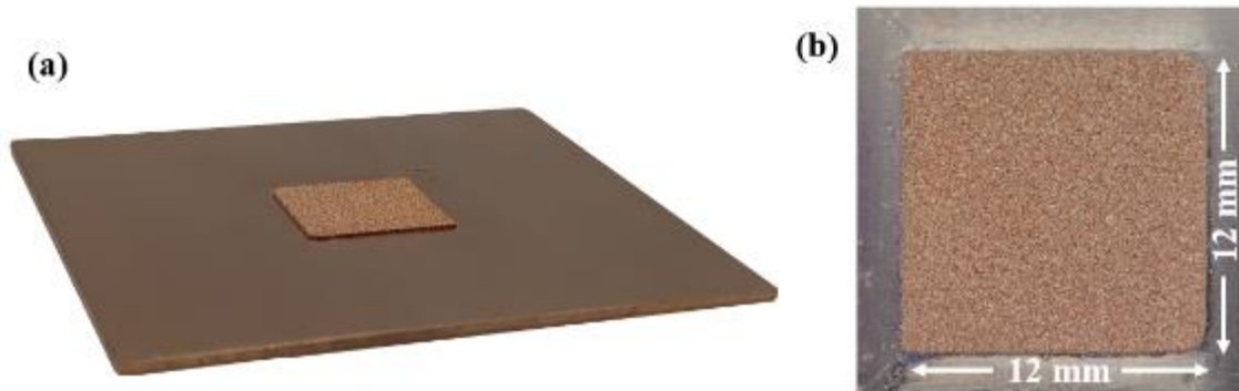
Figure 4.8. (a) Photograph of copper base with sintered copper wick at the center. (b) 89 \mu\text{m} average particle size wick
