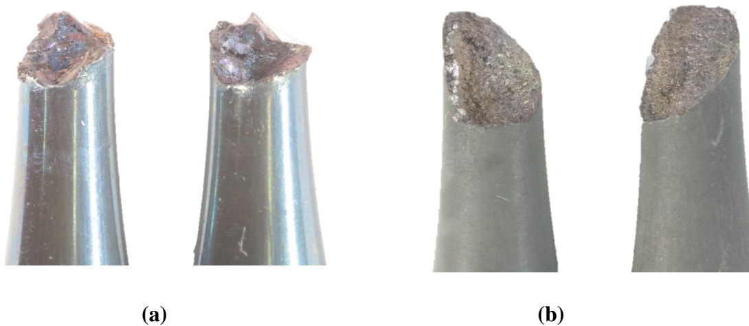
Figure 3.7. Comparison of fracture surfaces in torsional fatigue tests of Inconel 617 at 850°C: a) failed at N= 39.5k cycles b) failed at N=9.4m cycles
