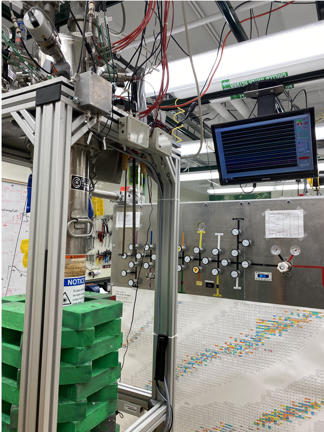
Figure 3.1. A picture of the ASTERiX detector, shielded with lead bricks. Vitalstatistix on the monitor screen and the gas system panel with valves are visible in the background.
