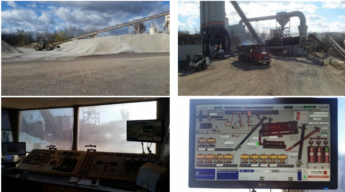
Figure 5.3. Hot-mix asphalt plant used to produce the control and test mixtures.
