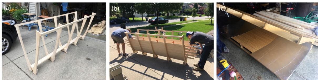
Figure 3.2. CPC construction process; (a) CPC skeleton with spines placed every 2 ft along the 8 ft section; (b) addition of the 1 in wide wood strips to create a curved inner CPC surface; (c) addition of aluminum foil for reflection and concentration of ambient solar irradiance within the CPC.
