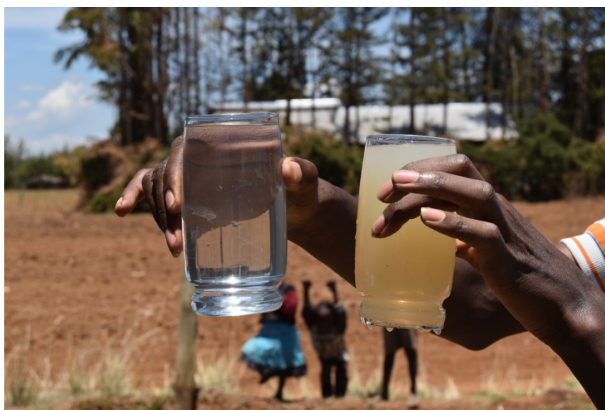
Figure 7.7. Water from the well at school D before (right) and after (left) treatment with alum.
