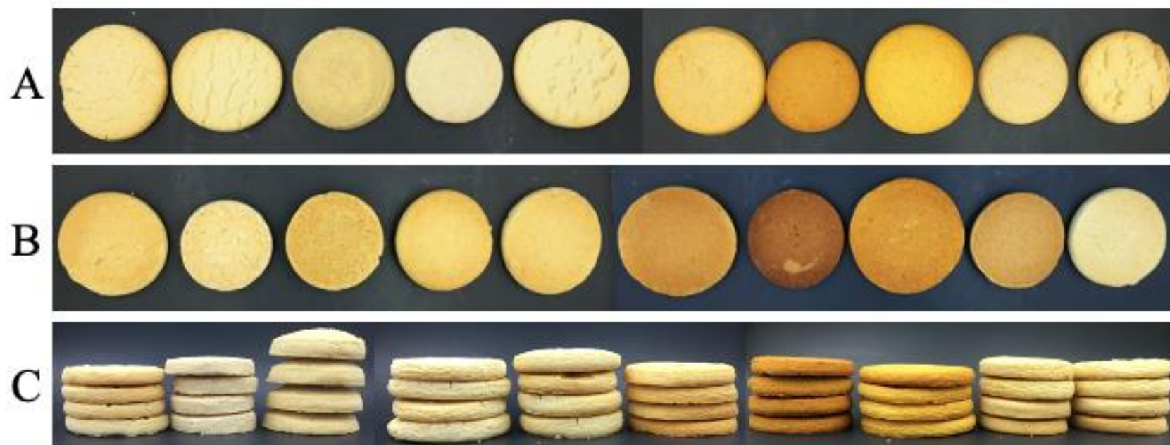
Figure 2-4 Top(A), bottom (B), and side view (C) of wire-cut cookies with various sucrose replacements (from left to right): sucrose, Miralax, Benefiber, maltitol, isomalt, IMO, allulose, FOS, HFCS, and amorphous sucrose.
