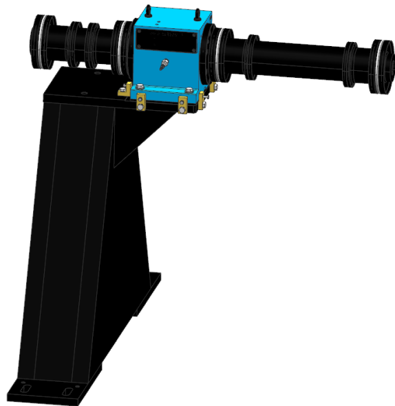
Figure 2.6. New driveline for the P3S facility consisting of flex couplings, torquemeter, and support structure.
