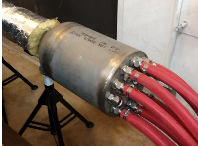
Figure 2.10. Redesigned orifice flow meter manifold.
