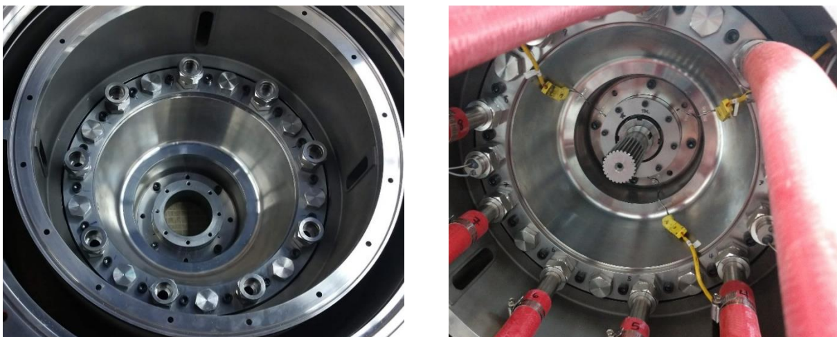
Figure 2.9. Redesigned rear plate for S3 cavity bleed flow with 18 symmetrically placed holes and a variety of plugs and open ports.
