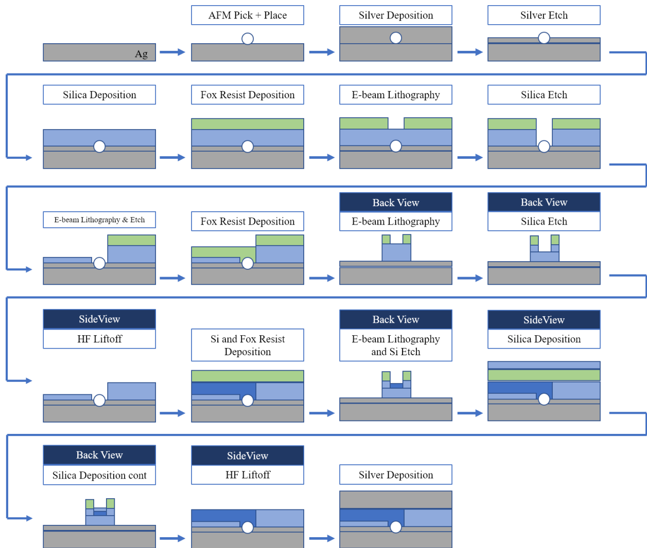
Fig. 4.6 Process flow for device fabrication. The device is fabricated using a combination of deposition of different materials in tandem with photolithographic techniques utilizing fox resist.
