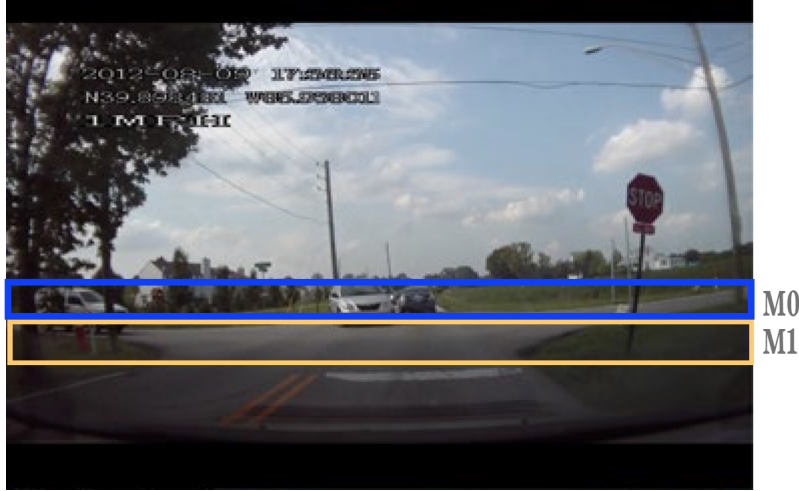
Figure 2.5. Example frame where zones or belts are set to average color there for motion profile images. M_0 is over the horizon in the frame to obtain traffic up to infinity, and M_1 is set for a closer range to finding surrounding vehicle motion.
