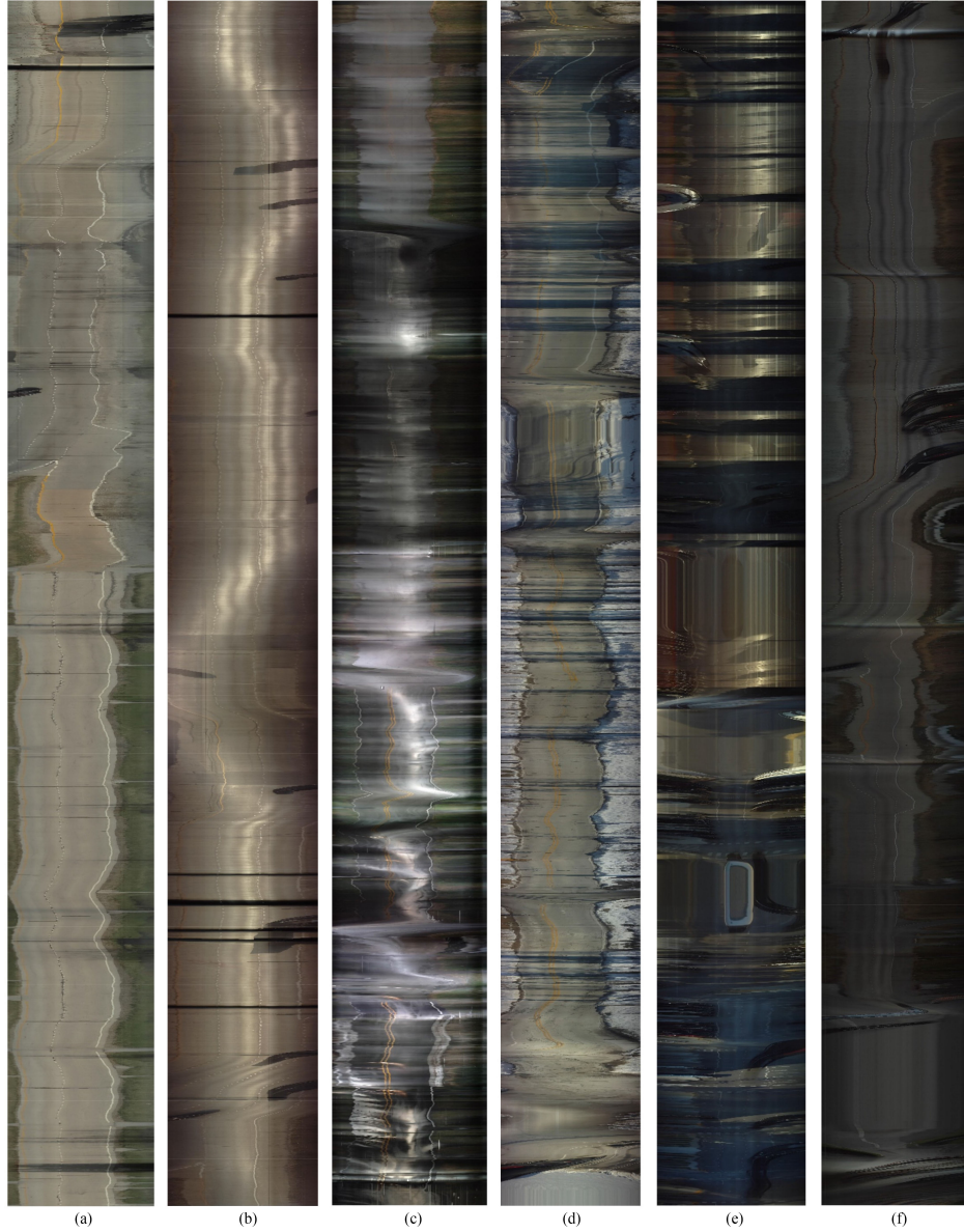
Figure 3.4. Road profile images captured in different weather and illuminations with time axes upward. (a) Sunny back to the sun with color roadside, (b) Sunny facing the sun with highlight on road, (c) Rainy on wet road with specular reflection of sky as highlight. Specular reflection is more dominant than road edges. (d) Snow-covered roadside with partial shadow, (e) Heavy shadow on urban road with road partly visible, and (f) dark lit. Road edge is barely visible.
