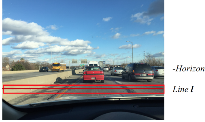
Figure 2.1. A frame from driving video. The relevant image area around the sampling line is also located to obtain the spatial attributes of the road, such as the linearity of the road edge.
