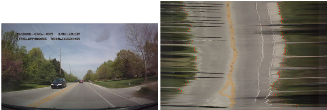
Figure 6.1. Road edges detected in road profile without using lane marks. Red bounded by two side green points are marked at road edges. High accuracy results in output outside road shoulder. Both passing vehicles (with the close-to-horizontal traces) and the road edges are located almost perfectly.
