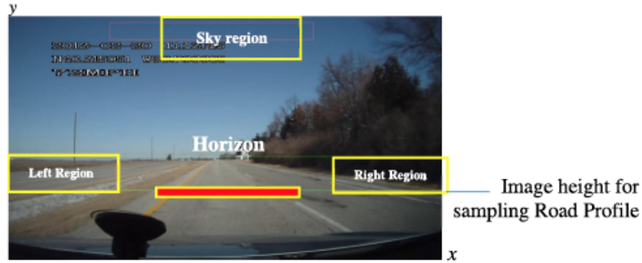
Figure 3.3. Four sampling regions in video frames for weather clustering. The averaged color in each region is recorded from every frame in the video.
