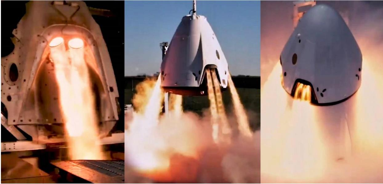
Figure 22. SuperDraco Engines firing during Crew Dragon Tests [54]
