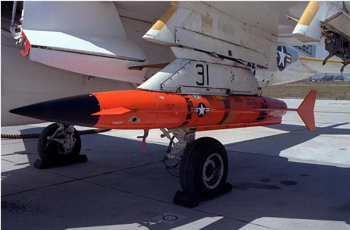
Figure 6. AQM-37A target missile loaded onto the wing of an A-6E Intruder aircraft [25]
