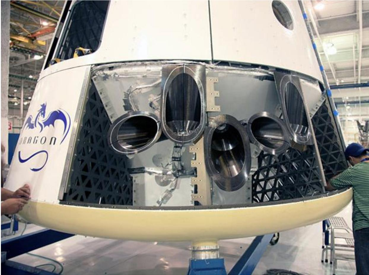
Figure 21. Draco Engine Nozzles on Dragon Qualification Unit [53]
