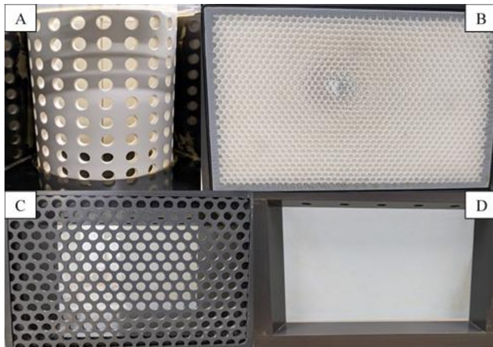
Figure 4-2 Flow conditioning sections. A is a PVC distribution pipe with 9/16” holes, B is the 3” long 1/4” Polycarbonate honeycomb and 24 mesh nylon screen, C is the 1/2” PVC perforated plate followed by a 34 mesh nylon screen, and D is the 44 mesh nylon screen
