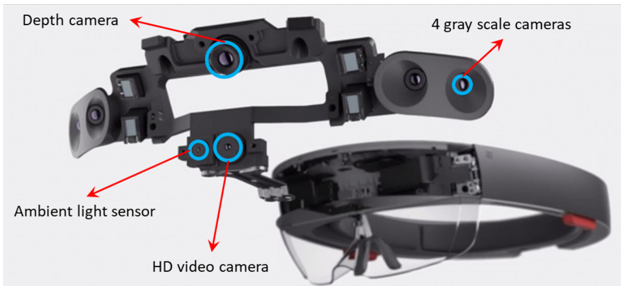
Figure 4.15. First generation Microsoft HoloLens. It is a head-mounted augmented reality device capable of RGB-D sensing.
