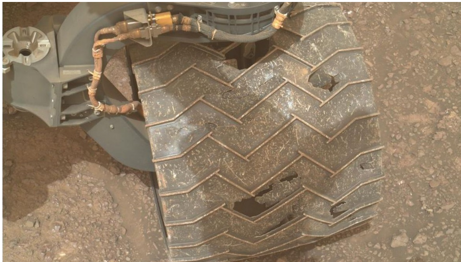
Figure A.2. Cracks on the rover wheel
