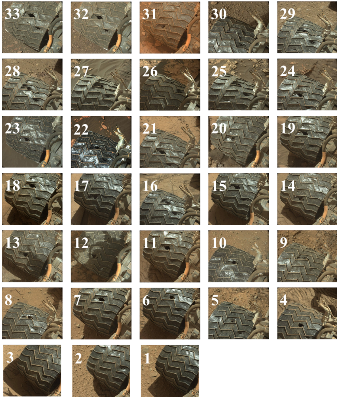
Figure A.6. A collage of identified corresponding images from various data acquisition rounds. The figure clearly depicts the time evolution of a crack under investigation in the reverse order. The figure legends represent the line-up of data acquisition rounds.
