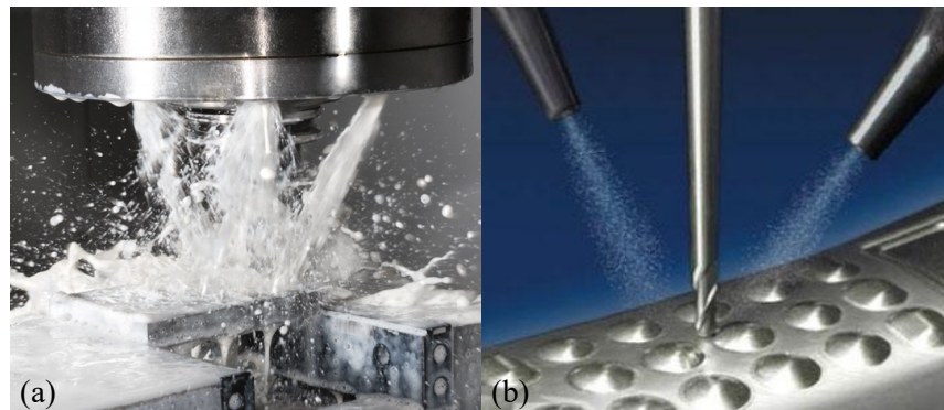
Figure 2.7 (a) Flood coolant [68], (b) MQL [69]
