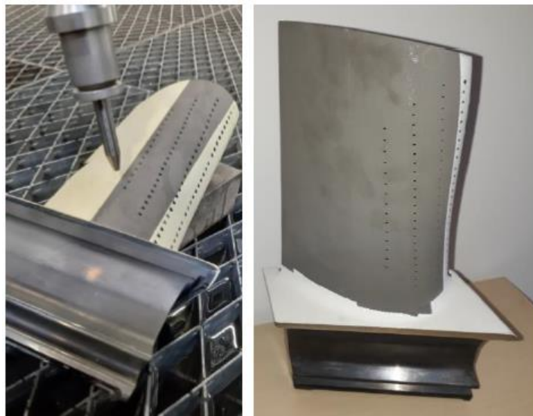
Figure 1.19. Waterjet stripping of TBC on a turbine blade [37].
