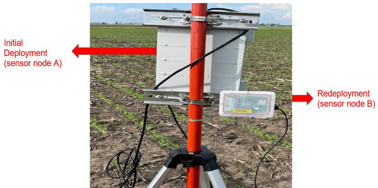
Picture 4.1: Initial deployment (sensor node A) & Redeployment (sensor node B)
