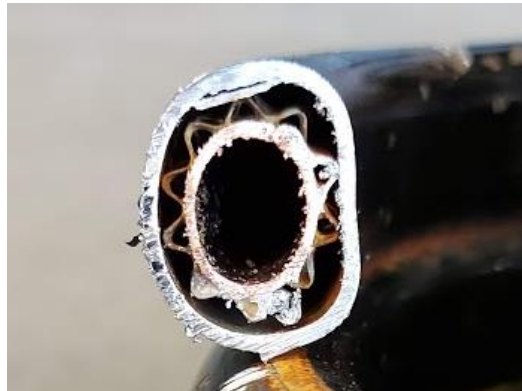
Figure 30: Inner tube and annulus of tube-in-tube evaporator with heat transfer enhancements (Brendel et al., 2022c).
