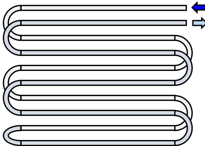
Figure 104: Schematic of evaporator coil for fin-tube heat exchanger.
