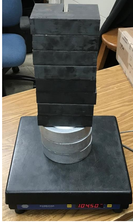
Figure 2-9: A picture of the calibration weights being weighed.
