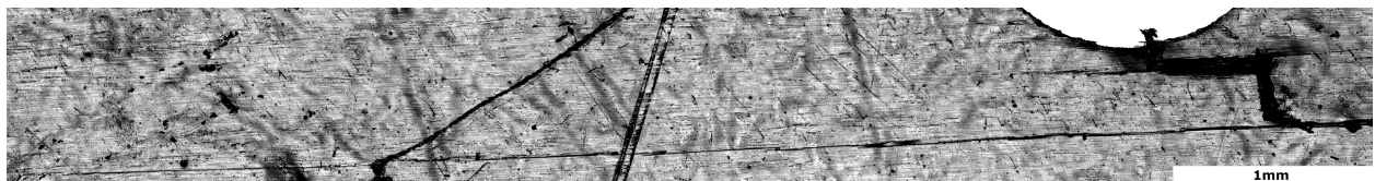
Figure 9.9. Lead crack emanating from buckled ply - Specimen 1-1-2
