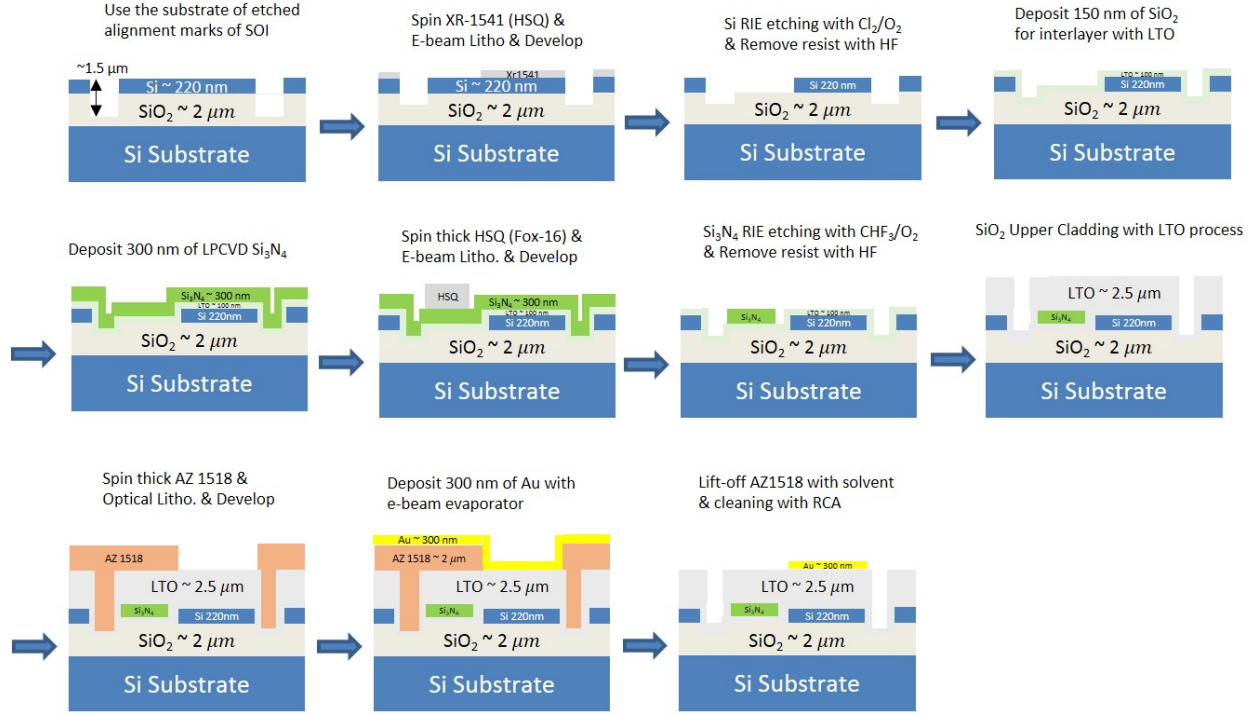
Figure 4.3. Fabrication process flow of silicon nitride to silicon waveguide array.
