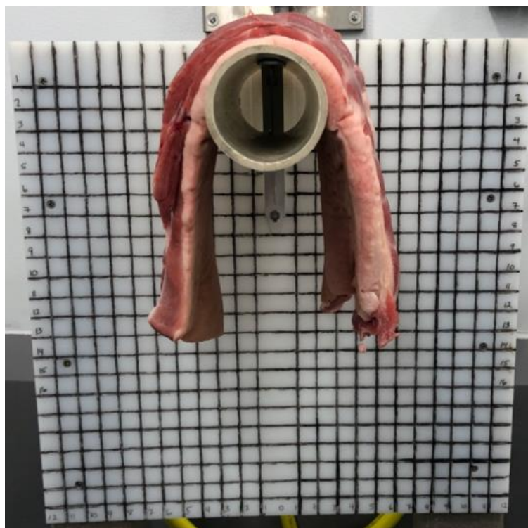
Figure 2.3 Belly firmness measured placing the boneless belly skin side down on a PVC pipe (diameter = 8.89 cm), with an X- and Y-axis grid. The distance between grid lines is 2.54 cm.
