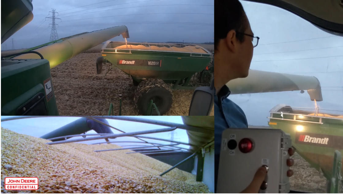
Figure 5.6. A representative frame in automatic unloading operation with Front to Back to Front fill strategy (associated with Visualization 11 )
