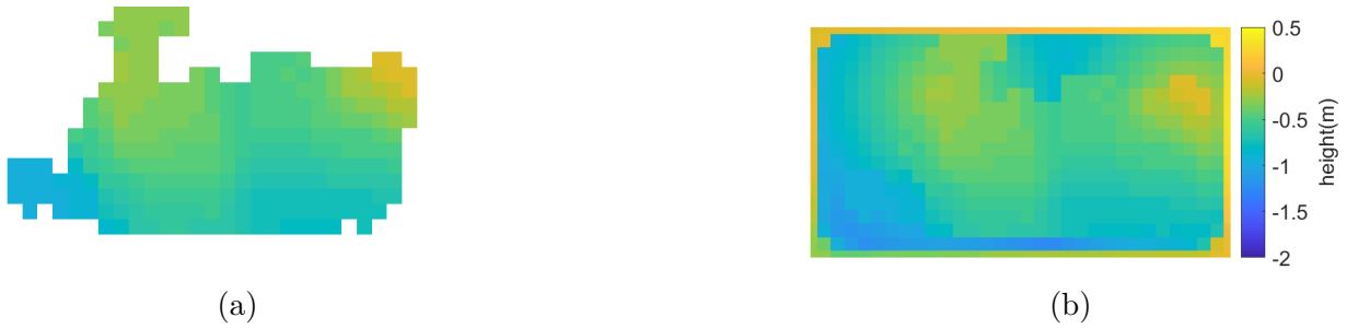
Figure 6.18. Initial profile estimation in the automatic unloading test (a) camera-based perception system feedback; (b) initial fill profile estimation.
