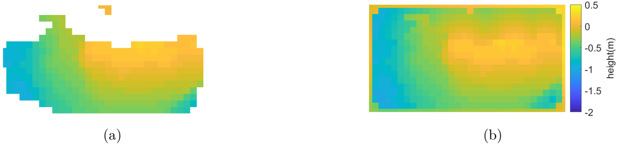
Figure 6.10. Initial profile estimation for manual unloading test: (a) camera-based perception system feedback; (b) initial fill profile estimation.
