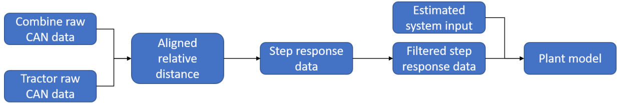
Figure 3.18. Data processing pipeline for experimental Machine Sync system ID
