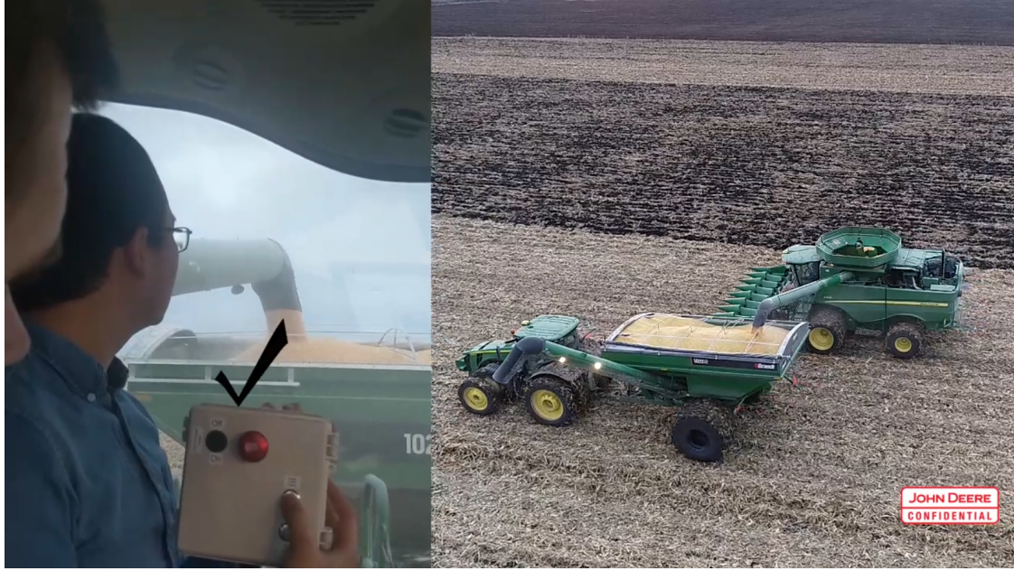
Figure 5.5. A representative frame in automatic unloading operation with Front to Back to Front fill strategy (associated with Visualization 10 )
