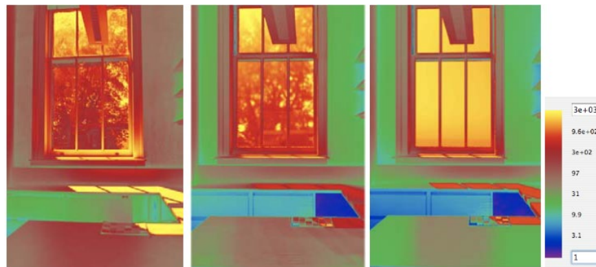
Figure 2.8 Comparison of the HDR image of the sky, IBL simulation, and generalized sky modelled simulation under clear sky conditions [88]
