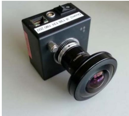
Figure 2.17 IcyCAM HDR vision sensor equipped with fisheye lens [48]
