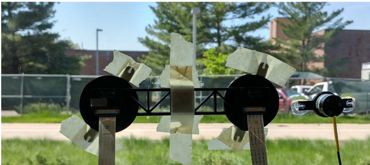
Figure 4.3 Fisheye stereovision sensor mounted attached to window
