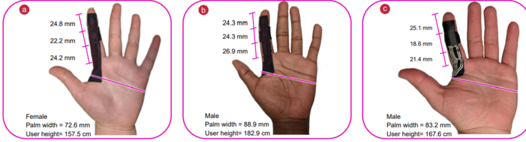
Figure 5.10. FabHandWear- Custom fit wearable design on different hands
