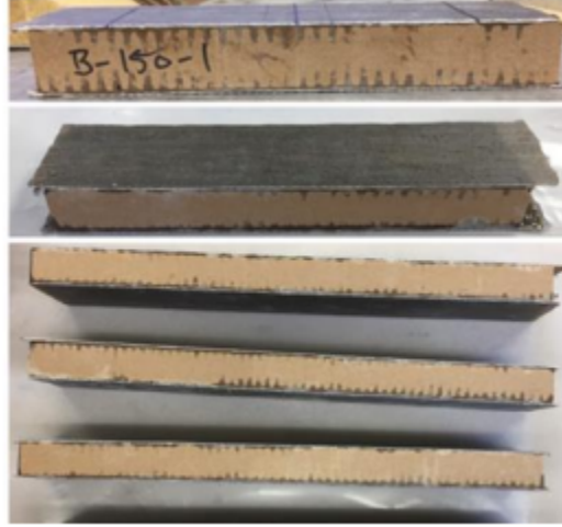
Figure 3.2. Corrugated cardboard core sandwich beams with bio based Flax Fiber reinforced composite skins [7]
