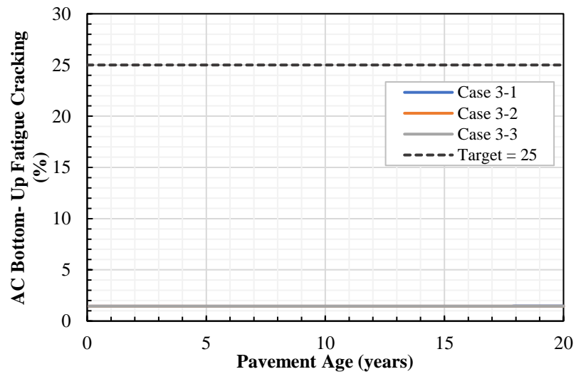
Figure 3.7 Development of IRI, rut depth, AC bottom-up cracking, and AC thermal cracking with pavement age (Cases 3-1 to 3-3).
