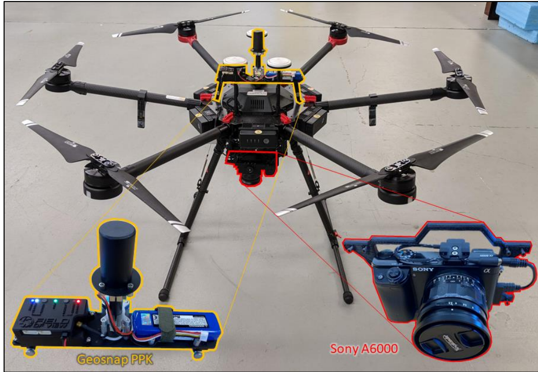
Figure 4. The UAS platform used in this study was a DJI M600 Pro (DJI, 2021) and was equipped with a Geosnap PPK (Field of View, 2021) which triggered a Sony A6000 Mirrorless Interchangeable Lens Camera (Sony, 2018).
