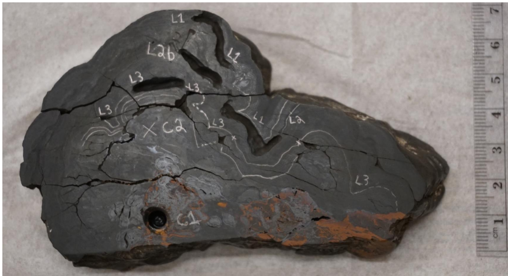
Figure A2.1: Sample NOD1: a botryoidal Mn-oxide nodule from Mine Bank Mine, VA. Traced layers are visible in pencil markings. NOD1-C1 is a drilled-out core from the center of the nodule. NOD1-L3, NOD1-L2b, and NOD1-L1 are layers that are further out from the core. NOD1-L1 is the rim. Note the oxidized iron near the center of the nodule, and the shiny erratic layers near the center that appear to cross-cut the concentric lamellae. These could imply that alteration has occurred after the initial precipitation of the nodule.
