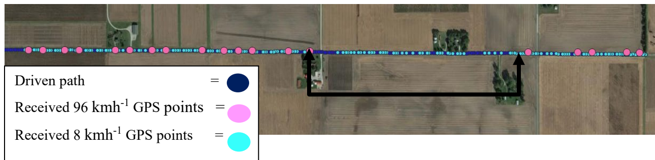
Figure 2.27: 8kmh -1 and 96 kmh -1 packet reception at 2400m
