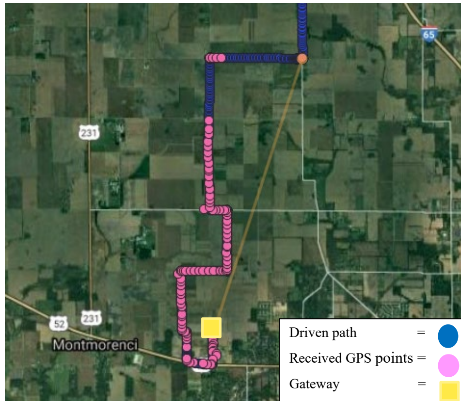
Figure 2.10: 7m gateway north bound testing with a max range of 7600m
