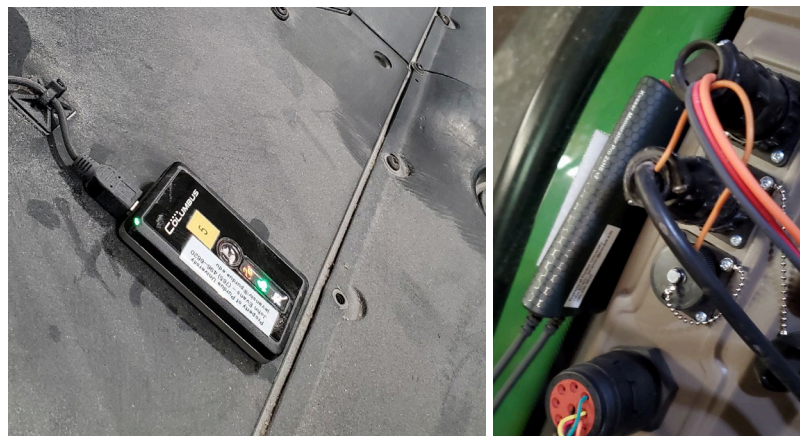
Figure 1.1: Columbus V990 Logger and Kvaser Memorator Pro 2x HS GPS Logger
