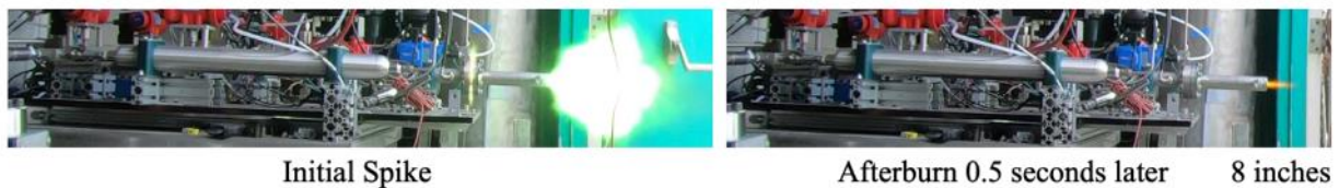
Figure 4.11: Initial detonation tube flame and secondary smaller flame as captured by a GoPro camera during Test 4
