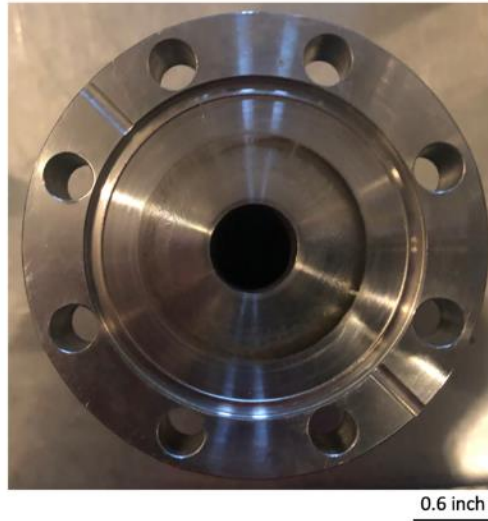
Figure 3.4: Knife-edge CF flanges used for sealing pressure in the shock tube
