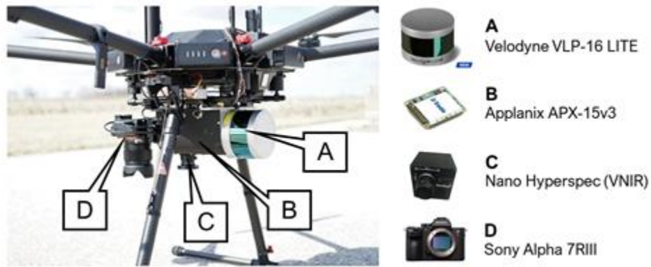
Figure 4.1 Unmanned aerial vehicle (UAV) used in this study. This system acquired hyperspectral, LiDAR, and RGB image. We use RGB data in this study.
