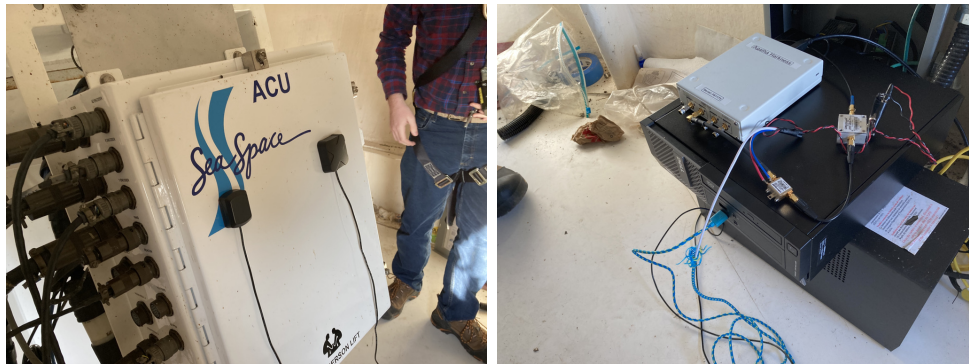
Figure 3.2. Receiver setup at Purdue. GPS and S band antenna mounted on the left. USRP, PC, and power on the right
