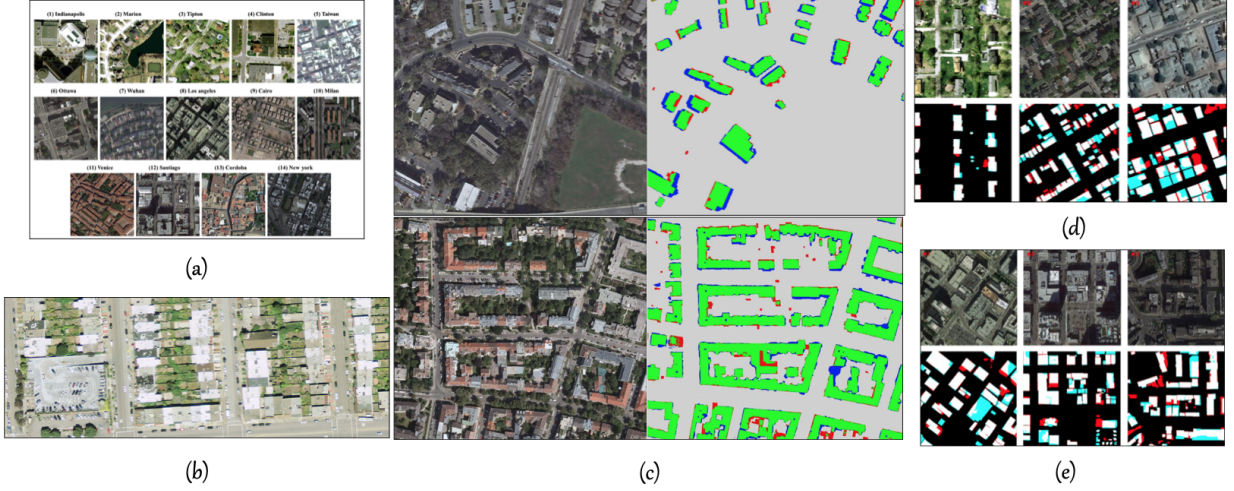
Figure 1.1. Illustration of some issues prevalent in current state-of-the-art building segmentation approaches. (a) Diversity in building appearance across the globe. (b) Similar spectral signatures of background and foreground pixels. (c) Errors mostly occur near the boundaries of buildings. (d) Errors due to occlusion from high vegetation. (e) Errors due to the presence of shadows.
