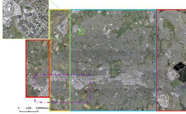
Figure 7.1. The WHU Aerial Building Dataset in Christchurch, New Zealand. The boxes in blue, yellow and red represent the areas used for creating the training, validation and test sets, respectively.
