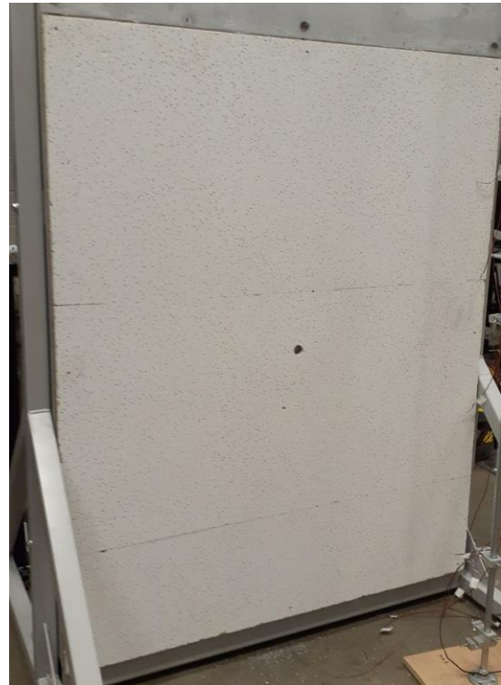
Figure 3.39 Ceiling surface treatment panel (Drywall acoustic tile)
