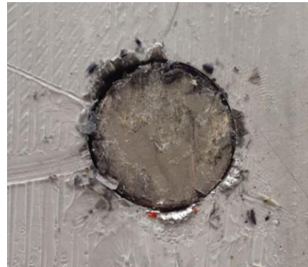
Figure 3.48 Magnets stuck in the slot hole in base panel
