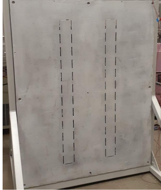
Figure 3.37 Aluminum base panel with guide slots in steel frame
