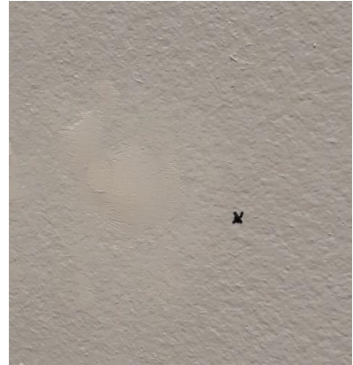
(c) Drywall after embedding sensor
