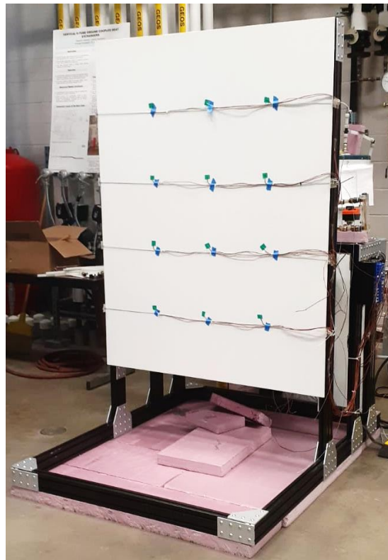
Figure 3.8 Test setup with front view showing surface thermocouple locations
