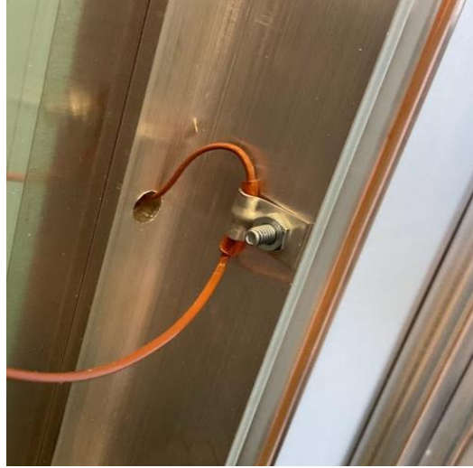
Figure 3.29 Welded-tip thermocouple assembly in final design
