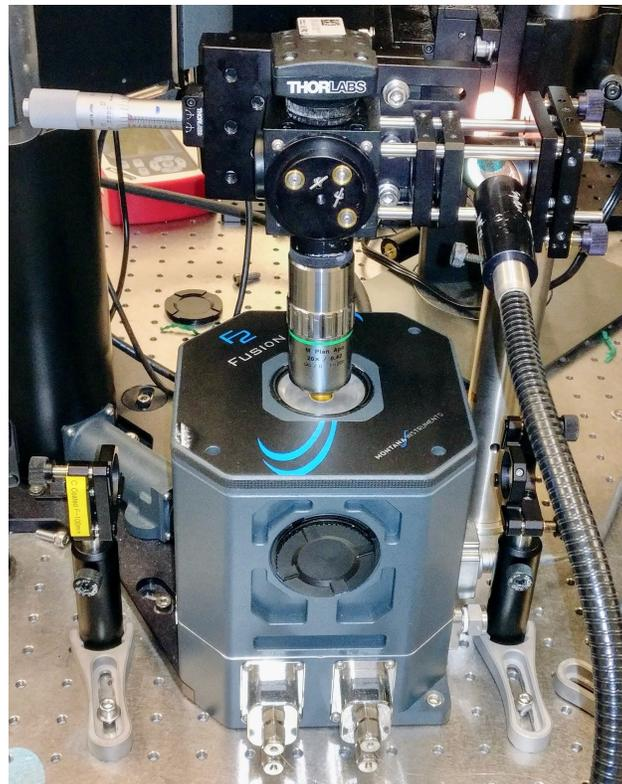
Figure 4.1. Cryogenic setup by Montana Instruments.
