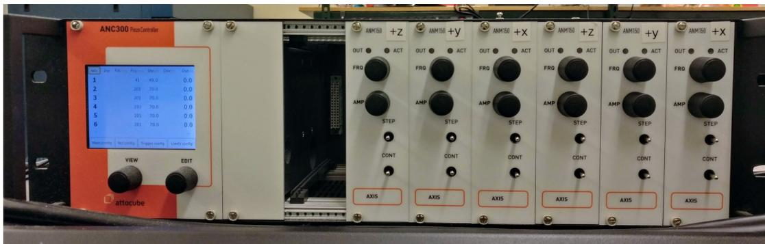
**Figure 4.3.** Controller for 3D nano-positioners for high-precision alignment for fiber-to-chip coupling.
