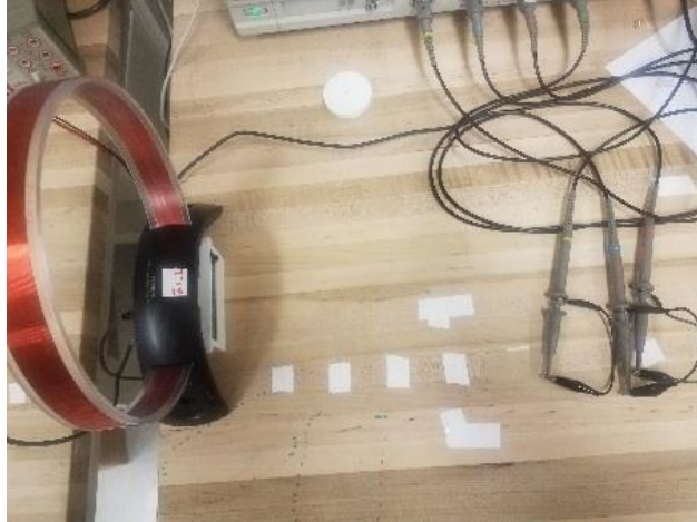
Figure 3.3.15. Oscilloscope null noise measurement test.
