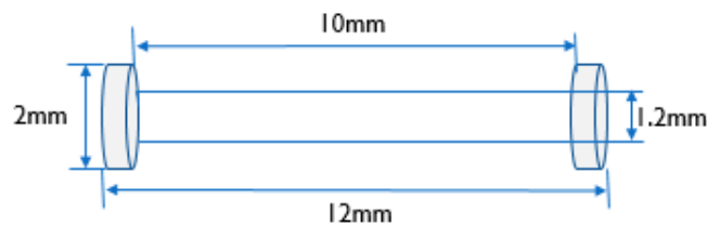
Figure 3.2.10. Plastic core for the proposed transmitter coil.
