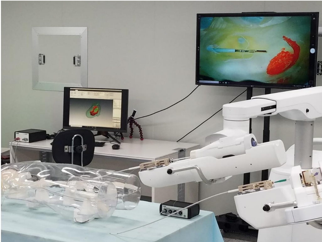
Figure 5.3.6. Point-cloud GUI representation of catheter tip and camera pointed at the tip.
