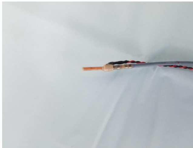
Figure 3.2.23. Transmitter coil (final version) attached to catheter tip.
