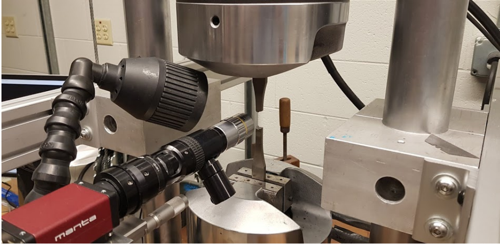
Figure 5.3. Camera configuration with 10x optical lens
