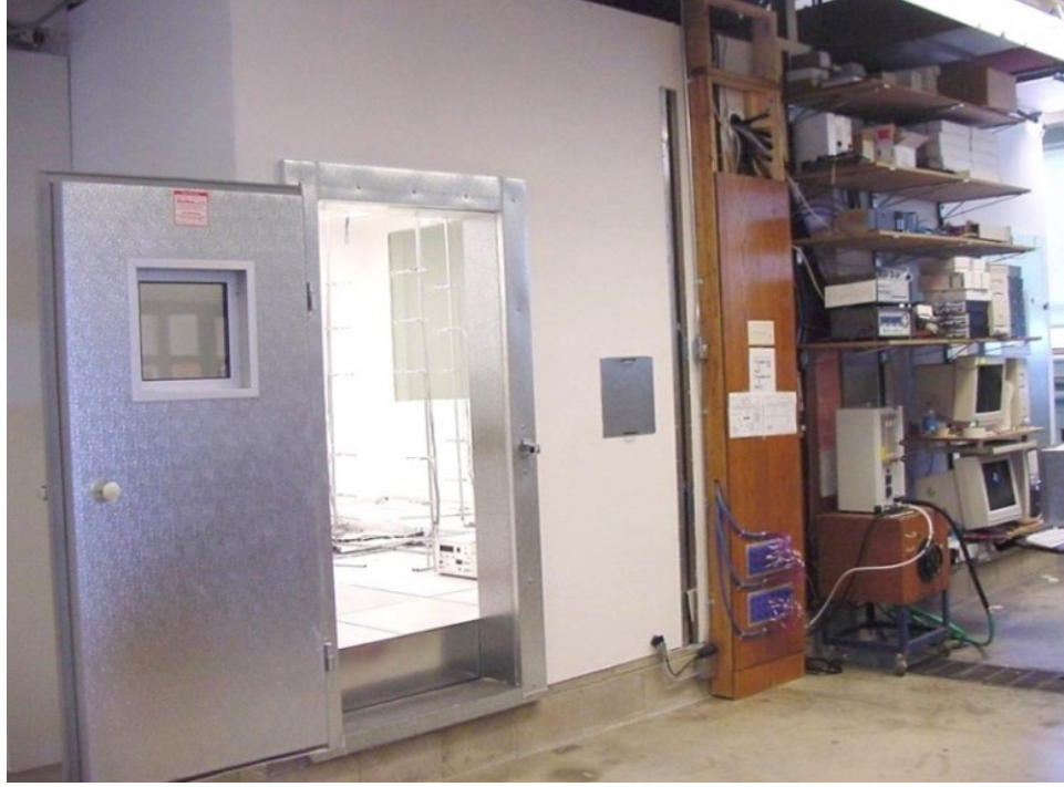
Figure 6.1. Indoor air quality chamber (IAQC) utilized for full-scale sensor testing.
