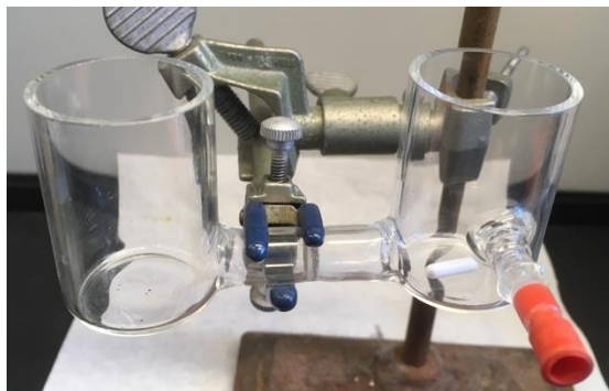
Figure S1. H-cell divided by a porous glass frit
