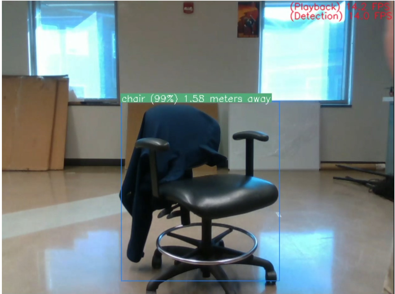
Figure 2.18. Screenshot of Real-Time Object Detection using MobilenetSSD-v2 at 720p Resolution
