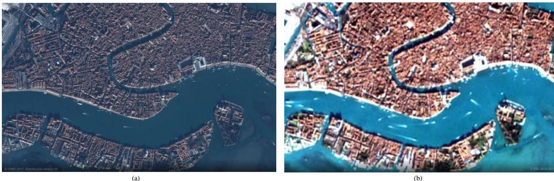
**Figure 1.1.** *Two Satellite Images of Venice.* (a) A 50cm high-resolution image from Pleiades satellite (Airbus). (b) A 10m per pixel medium-resolution image from Sentinel-2.
