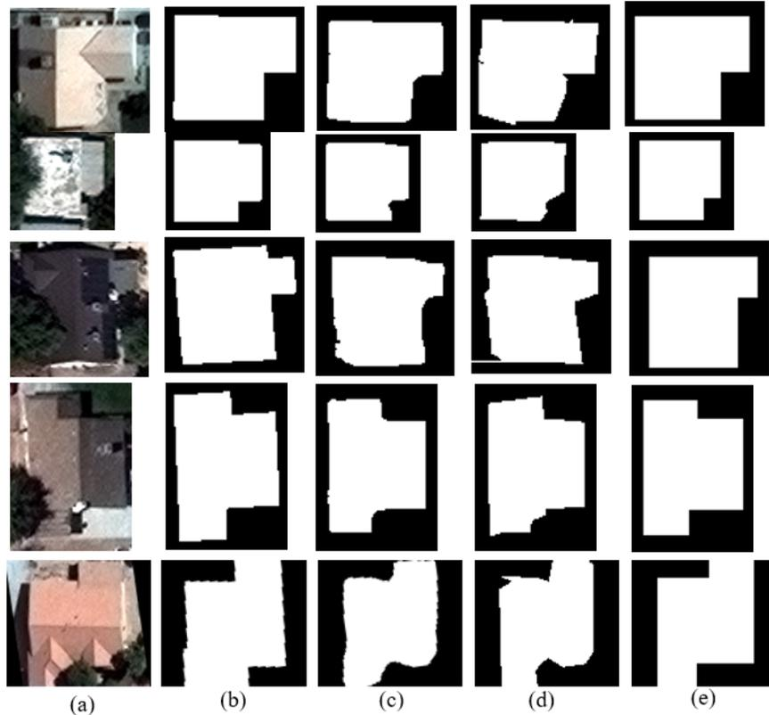
**Figure 7.15.** *Qualitative Comparison.* (a) Real images. (b) Ground truth footprints. (c) Initial building footprint segmentations. (d) ASIP results. (e) Our results.
