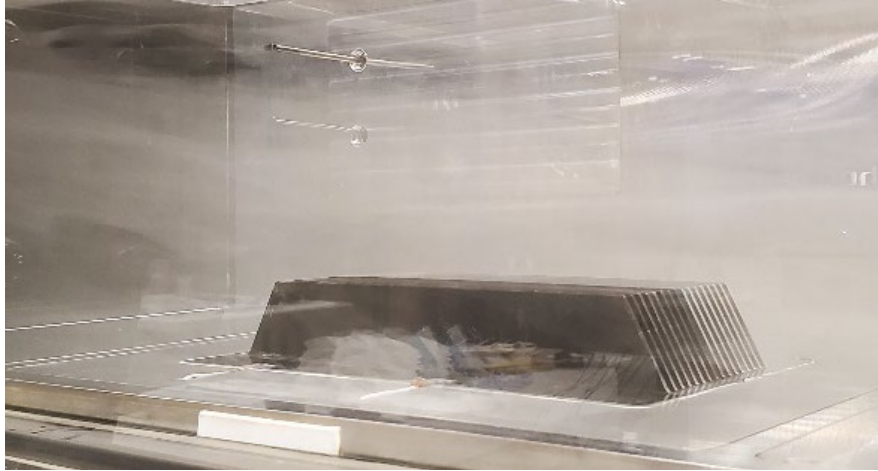
Figure 2.8 Smoke Generated at No-Flow Conditions over the Baseline Fin Design
