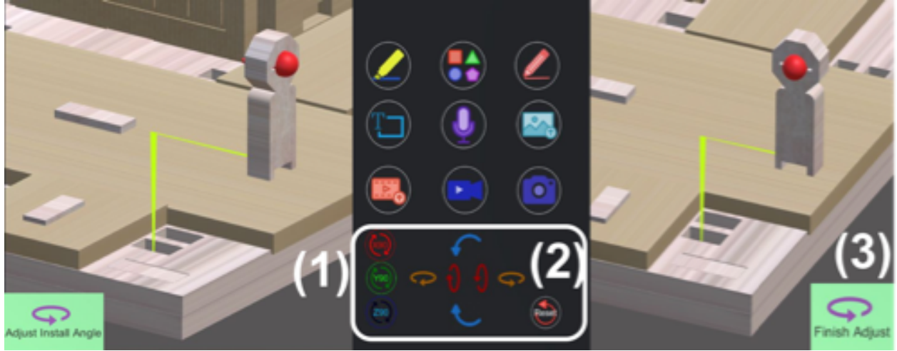
Figure 2.5. Angle adjustment process: (1) Object A and path have the wrong orientation; (2) Angle Adjustment tools can be used; (3) Object A and path are aligned. Sample objects from our mini smart-city user study.
