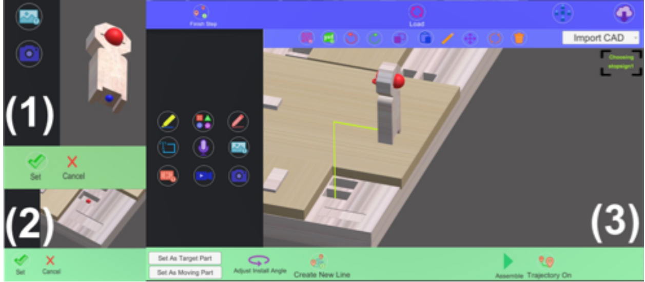
Figure 2.6. Creating Animation Process: (1) select start point from Object A and set; (2) select finish point from Object B and set; (3) path is generated and instructor can preview animation.
