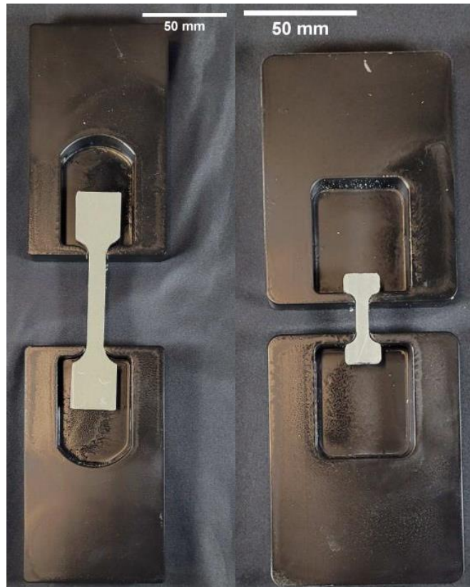
Figure 3-5. Fixed Grips Designed for Tensile Tests with JANNAF (Left) and Micro (Right) Sizes.
