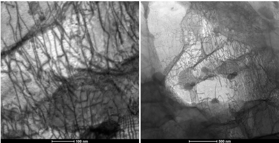
Figure 4.3. BFSTEM images of PM-HIP unirradiated sample.
