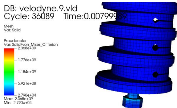
Figure 4.7 Pseudocolor plot of Von Mises Criterion of the bottom of the neck. Top elements of neck bold can be seen to have a higher value than surrounding elements.
