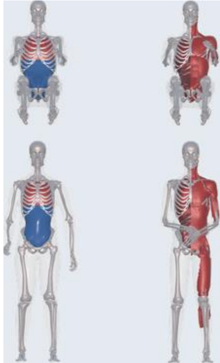
Figure 2.1 Simplified seated and standing GHBM 50 th percentile male models (left) and detailed seated and standing model (right). Figure from [49].
